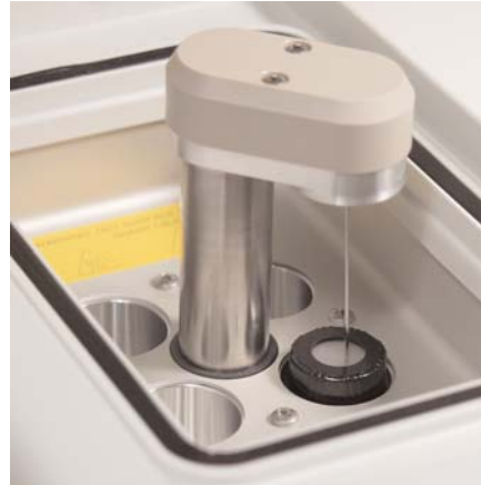
The oven accommodates four standard 40-ml vials. Needle can be easily inserted for withdrawing the sample.
